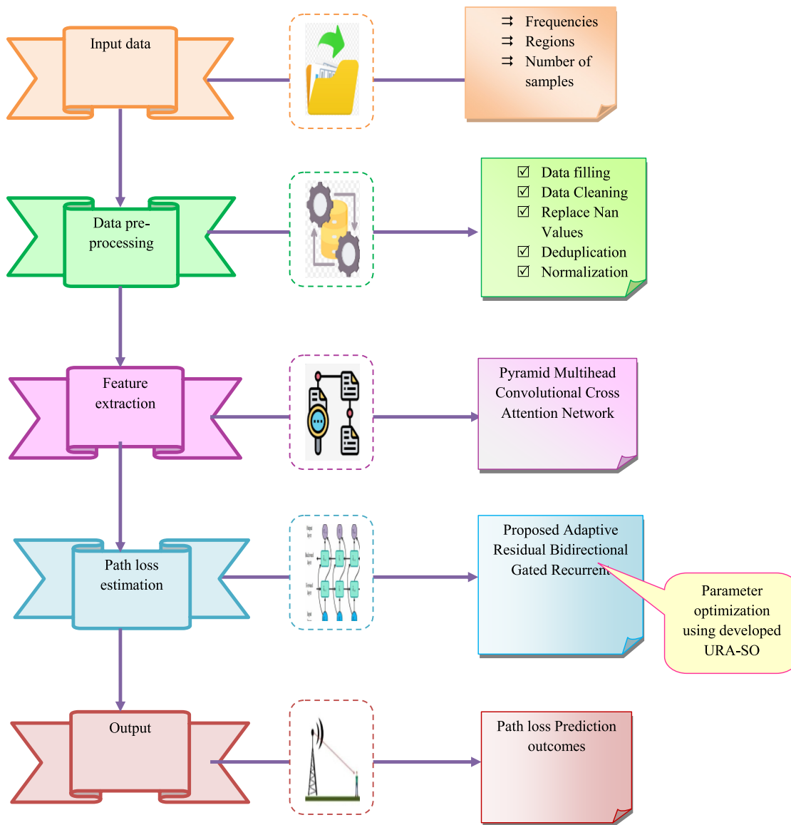
FIGURE 1 | Architectural framework of the proposed path loss estimation model in mm-Wave communication.
